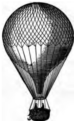
FIG. 39. A balloon floats in the air somewhat as a cork floats in water.
